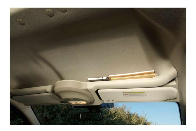
The overhead storage above the driver's head can accommodate a variety of objects in a volume of up to 12.5 litres, which also locates the sun visors and the courtesy light. Openings placed at the rear of the overhead storage make it possible to see stored objects and retrieve them more easily.
