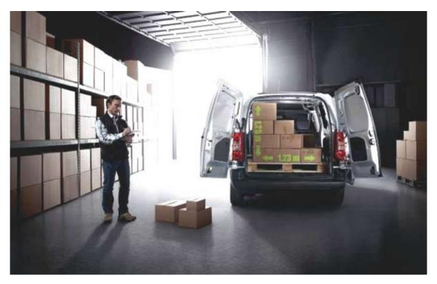
At the rear, the asymmetric hinged rear doors can accommodate a load with a maximum width of 1250 mm and a height of 1200 mm. The square shaped loading space helps to facilitate loading and unloading. The hinged rear doors can be opened out to an angle of either 90° or 180°, making loading operations much easier.
