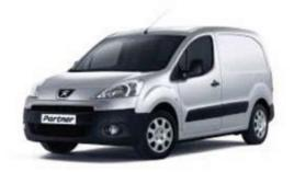
The new Partner is available in two body styles with a length of 4.38 metres and 4.63 metres, on a single wheelbase of 2.73 metres.
